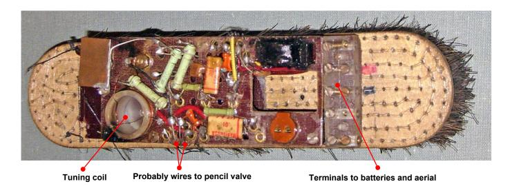
Bottom half of the broom with the RF transmitter, microphone and modulator
